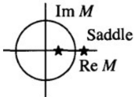
Fig. 4.7. Characteristic multipliers in the complex plane. If both multipliers lie within a circle of unit radius (the unit circle), then the corresponding limit cycle is stable. If one (or both) of the multipliers lies outside the unit circle, then the limit cycle is unstable.
