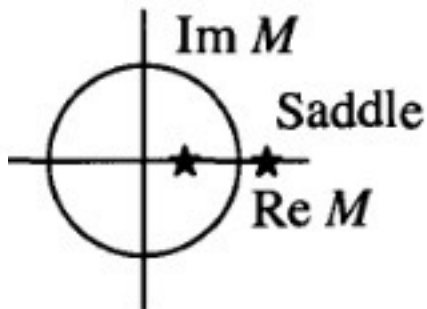
Fig. 4.7. Characteristic multipliers in the complex plane. If both multipliers lie within a circle of unit radius (the unit circle), then the corresponding limit cycle is stable. If one (or both) of the multipliers lies outside the unit circle, then the limit cycle is unstable.
